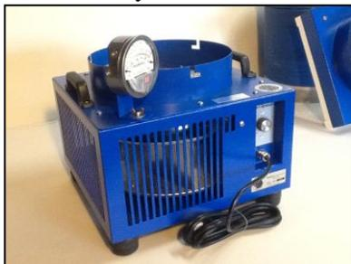
3. If the pressure measurement on the gauge remains at less than 0.4 inches of water column with the impeller running at maximum RPM, additional sealing of the RV should be examined. A major release of air pressure will usually be evident by inspecting all exterior components on the RV. *(Look for open or unsealed vents, doors, or hatches indicated by outrushes of air. Check for a range hood vent that is unlatched or dry sink traps)*
