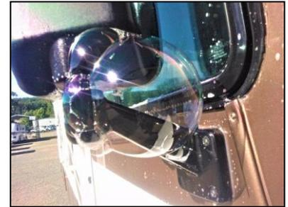
7. Repair all sources of air leaks. If air pressure can escape, moisture can enter!
