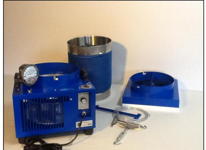
7. Insert duct cuff into bottom fan assembly. Secure with twist lock.
